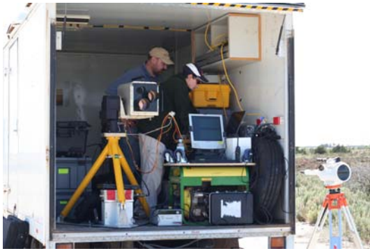
Figure 21 Interrogator in the instrumentation van. Scintillometer receiver at right.
