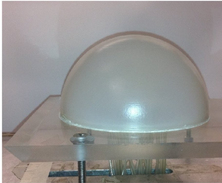
Figure 1. Photograph of our hemisphere mounted on an elevated surface in the wind tunnel without the plasma actuator.
