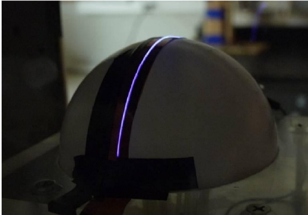
Figure 3. Photograph of the light emitted by the plasma actuator mounted on the hemisphere in the wind tunnel.
