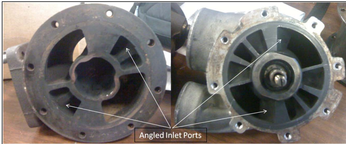
Figure 39: Angled inlet ports on Comprex® pressure wave supercharger
