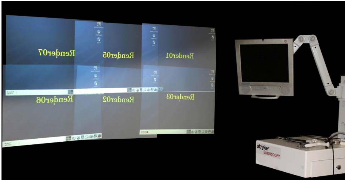
Figure 7. A prototype six-projector display in our visualization lab. The overlap among the images is made visible in order to show the contribution of the individual projectors.
