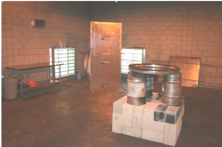
Burn Room With Elevated Burn Pan and Fuel Tank Behind Radiant Barrier
