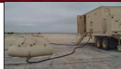
3000 GPH ROWPU for EAD (2,000 GPH on salt water) (shown with 3000 gal onion tank )
