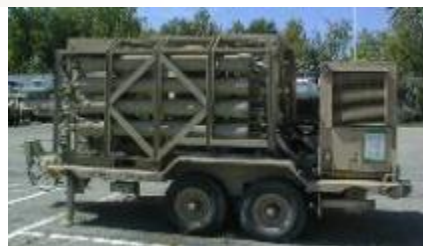
600 GPH ROWPU for Divisions and below (600 GPH on Salt water)
