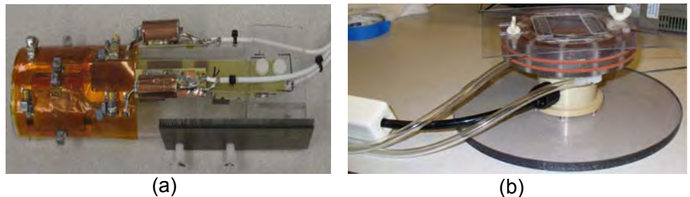
Figure 4. An MRI coil (a) was built for mouse imaging on Philips 3T scanner. A mechanic stage (b) was constructed for holding/stabilizing the mouse and the coil within the MRI scanner. Inside the stage, water will be used as the interface between the HIFU transducer and the animal.
