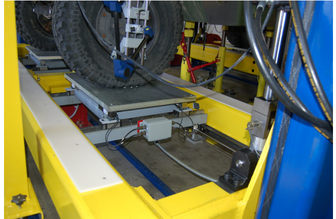
Figure 2: A typical wheel pad. The top plate and the heavy plate supporting the load cells are visible. The linear rails allowing longitudinal and lateral motions are visible. The crossed roller bearing allowing steer motion is not visible in the photograph, but it is between the top plate and the load cell plate.
