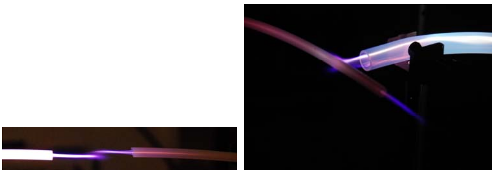
Figure 13. The images show the previously observed ability of the plasma plume of a powered sample to induce a plasma within the tubing of an unpowered sample with He gas flowing.
