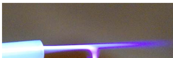
Figure 14. A close-up of the plasma plume being divided when scissors are held close as a local ground.
