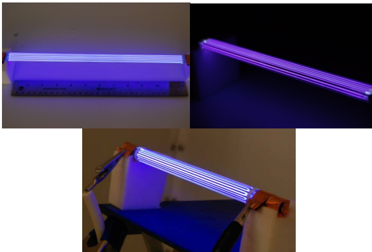
Figure 6. Cap-DBD in air: 12'' planar, 1x10, 250 \mu\text{m} gap width (left); 6'' 3-D, 3x6, 250 \mu\text{m} gap width (middle), 12'' cylindrical, 20 tubes, 0 \mu\text{m} gap width (right).
