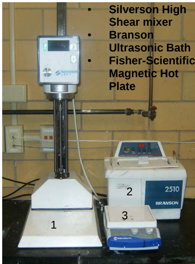
Figure 3. Image of mixing apparatus' including: 1. Silverson high shear mixer, 2. Branson ultrasonic bath and 3. Fisher Scientific magnetic hot-plate.
