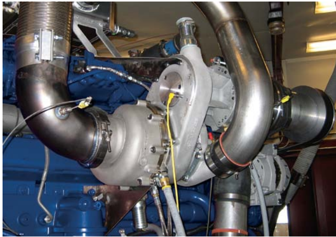
Figure 4: Current generation large diesel SuperTurbo
