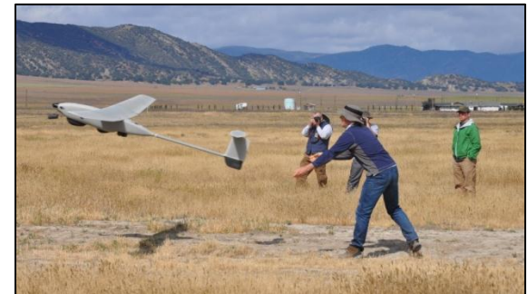
DARPA funded, fuel cell powered UAV (22 lbs). Photo courtesy of Lockheed Martin.
