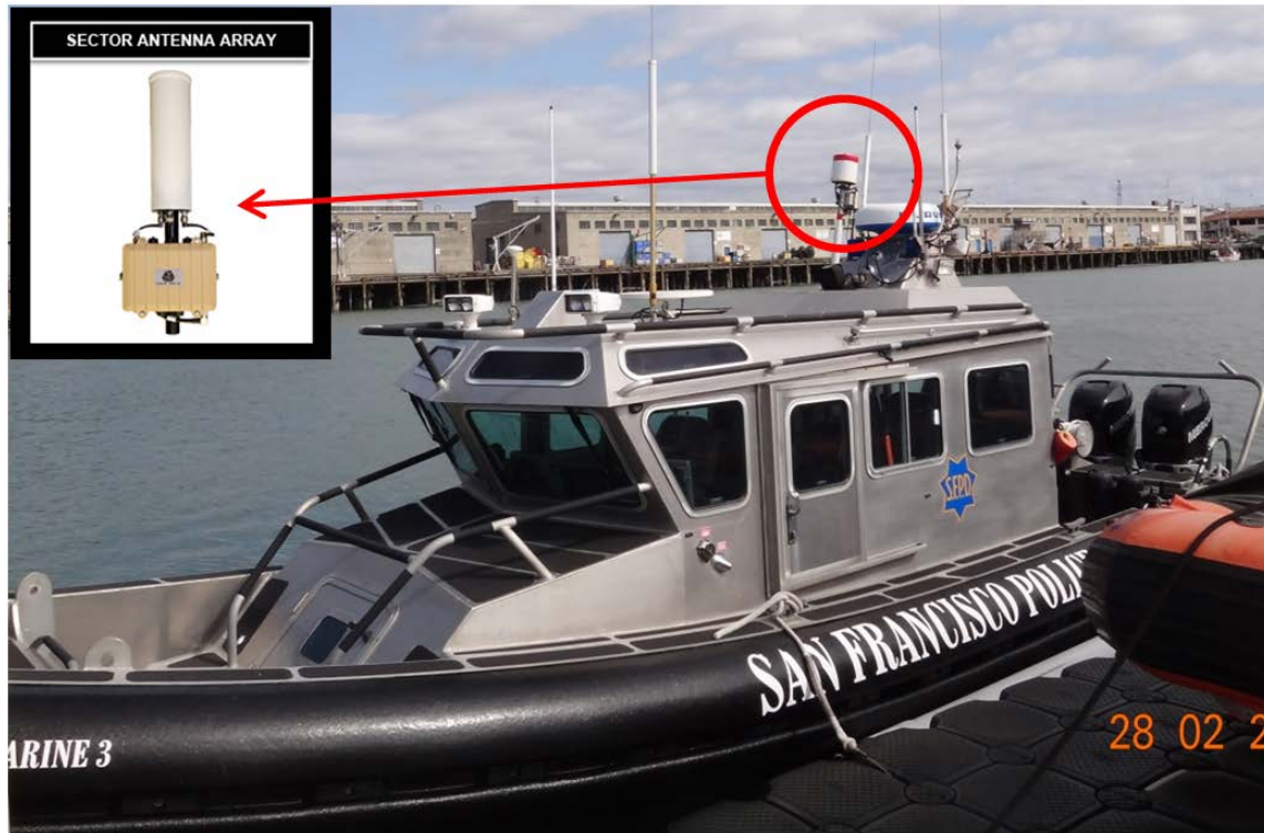
Figure 6. Sector Antenna Array and Quad Radio Router
