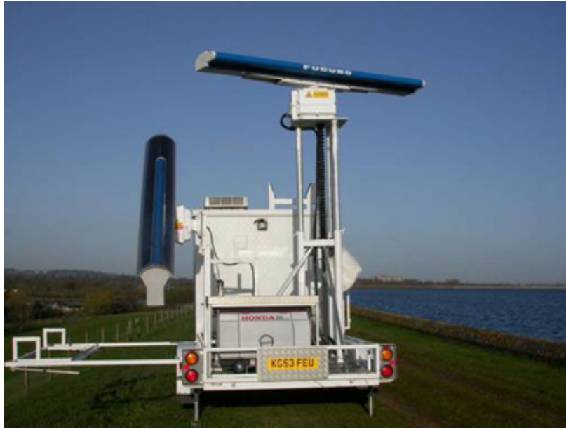
Figure 29. Mobile Surveillance Radar (Image from Mathworks website)
