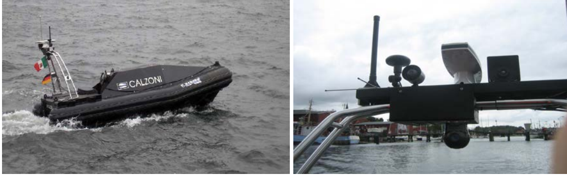
Figure 21. USV U-Ranger *7 and sensor suite (From [47])
