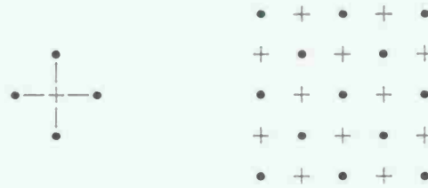
FIGURE 6.1. The four-element cross-neighborhood and the tessellation of the index set \mathcal{S} into two disjoint sublattices \mathcal{S}_e and \mathcal{S}_o .
