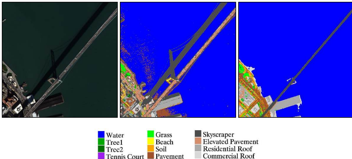
Figure 44. The San Francisco-Oakland Bay Bridge: left–true color; center-MSI classification; right-fused classification
