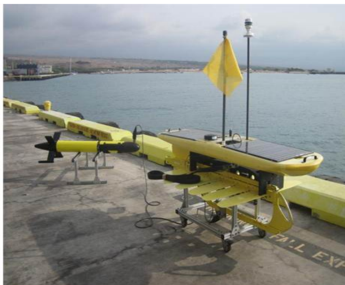
Figure 2.6: Pierside with a Wave Glider and tow body provided by LRI
