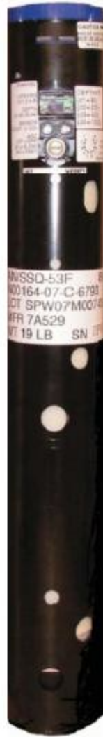
Figure 7. AN/SSQ-53F DIFAR Passive Sonobuoy (From Sonobuoy Tech Systems, 2008)
