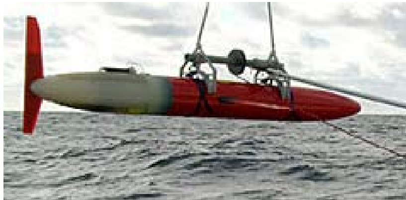
Figure 27. Spray Glider Launch w/Strap & Davit from (Krupski, 2012)
