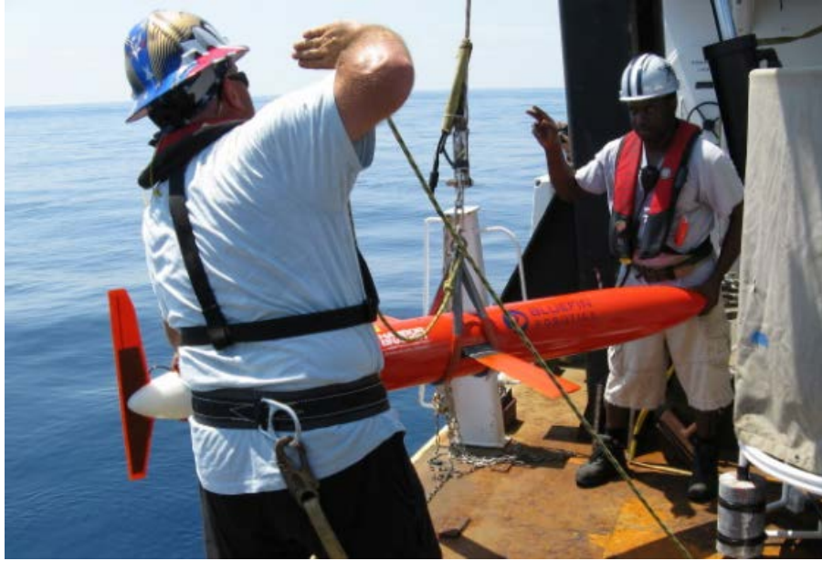
Figure 27. Spray Glider Launch w/Strap & Davit from (Krupski, 2012)
