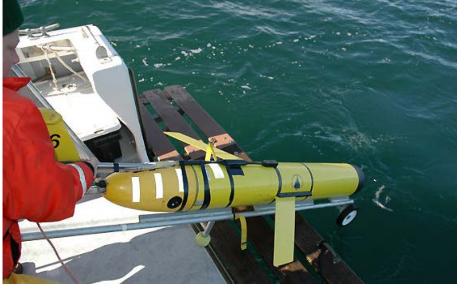
Figure 29. Slocum Electric Launch from Surface Ship Guide Rails from (Quest Marine Services, 2007)
