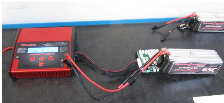
Figure 66. battery connected to balancer and charging
