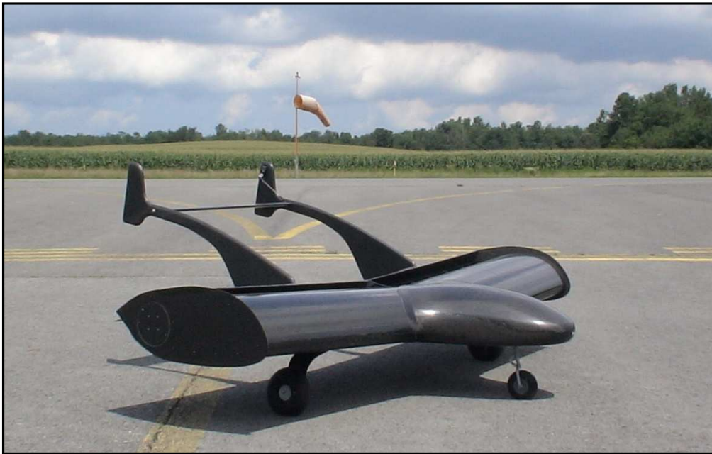
Figure 3. First working prototype of a CFF-propelled air platform by Propulsive Wing, LLC
