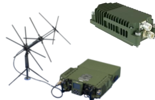
Manpack with MUOS Appliqué and Antenna
