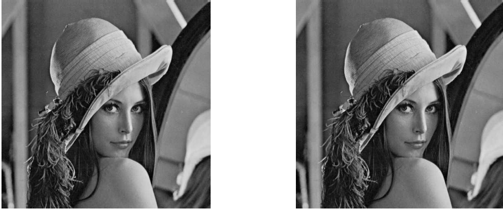
Fig. 12. Left: An image compressed using the SPIHT algorithm at a bit rate of 3 bits per pixel before the use of entropy coding. Right: The same image after anti-forensic dither has been applied to its wavelet coefficients.
