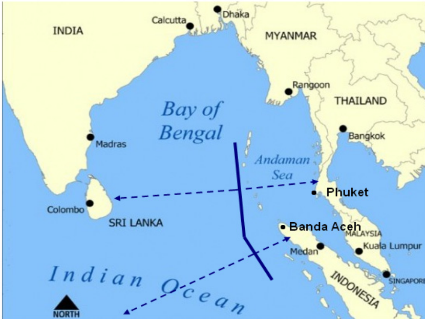
Figure 6. Propagation geometry of 2004 Indian Ocean tsunami showing the two major faultlines and propagation along their perpendicular bisectors (adapted from phuket.news.com).
