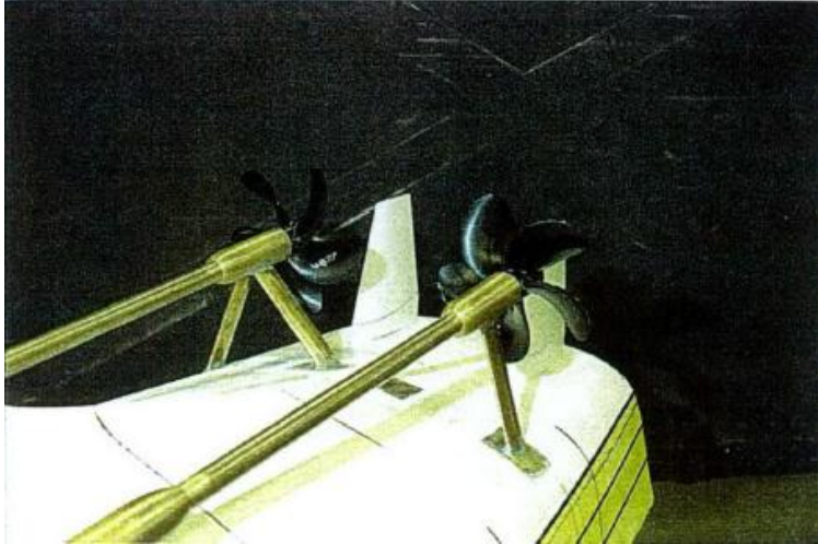
FIGURE 17-DTMB 4876 AND 4877 PROPELLERS ON DTMB 5415 MODEL (REPRODUCED FROM [19])
