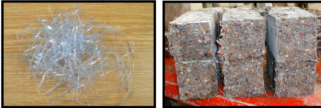
Figure 14. PET fiber and test blocks from Vytlačilová study.
