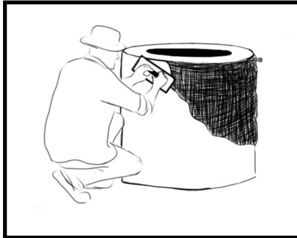
Figure 37. External FRBM Finish applied to mesh
