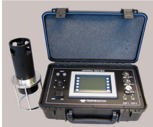
Figure 26. UDB-9400 Universal Deck Box, including its deployable transducer (left) (from [5]).
