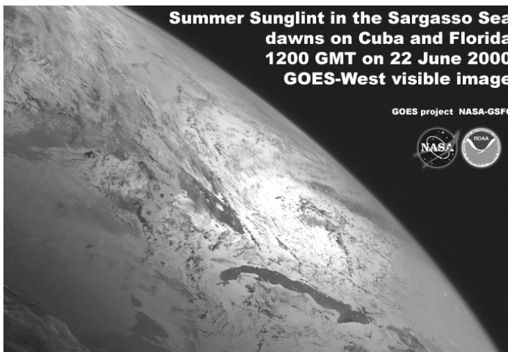
Figure 12. Another example demonstrating the effect of sun glint on the imager (image captured by the GOES satellite on 22 June 2000) (Image from http://rsd.gsfc.nasa.gov/goes/text/hotstuff.html )
