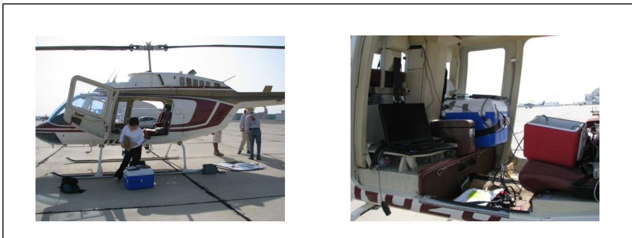
Figure 21: Spectroradiometric Measurements Using Low Altitude Flight
