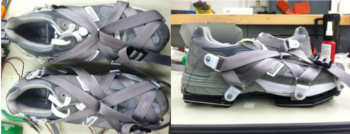
Figure 19: Binding system for force sensor to shoe. A “dummy” sensor made of plastic was also produced to provide symmetry to the other foot for the normal subjects.
