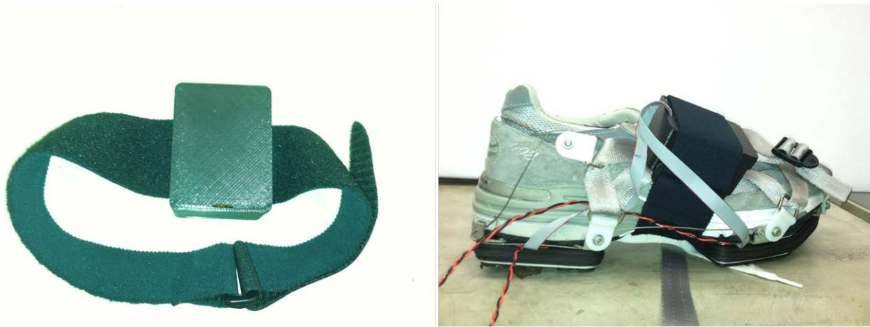
Figure 12: Enclosure and velcro strap for individual sensor boards which go on either the foot or limb segments (right) and enclosure with sensor board connected to the F/M foot sensor attached to the shoe (left).
