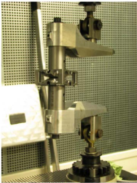
Figure 16: Test setup for smart pylon F/M sensors
