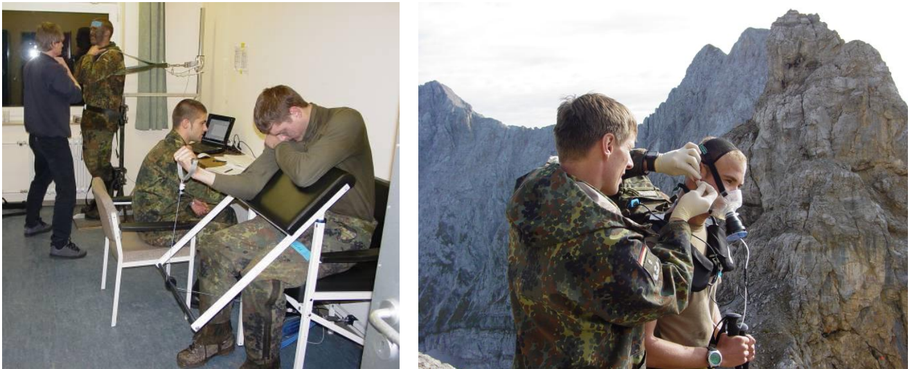
Figure 2: Data collection in the field: Strength measurements (elbow flexor and trunk flexor) after MOUT exercise (left); Blood lactate concentration, oxygen uptake, ventilation, heart rate during mountain march (right)
