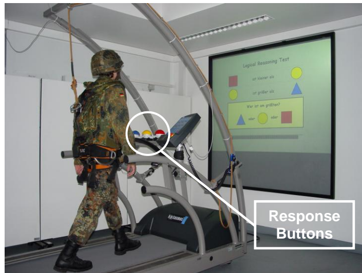
Figure 6: Experimental set-up during the first march phase ("Plain"). The three different coloured response buttons are mounted in front of the participant.
