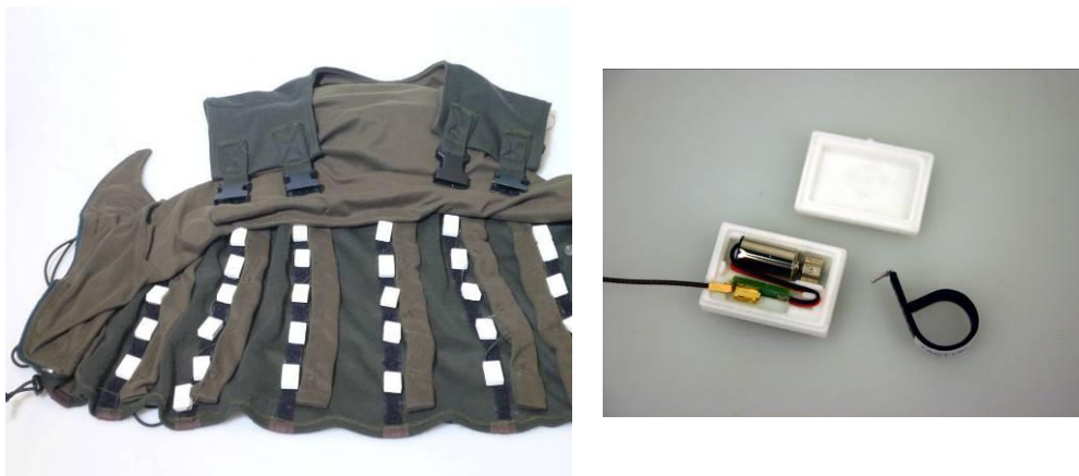
Figure 3: TNO Tactile Torso Display (left) and inside view of tactor (right).
