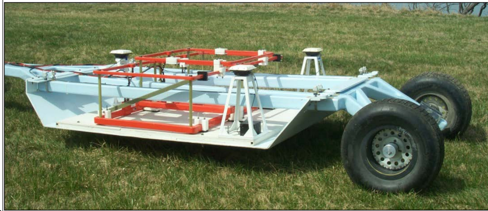
Figure 4-3 Close-up of MTADS EM61 array with GPS and IMU.
