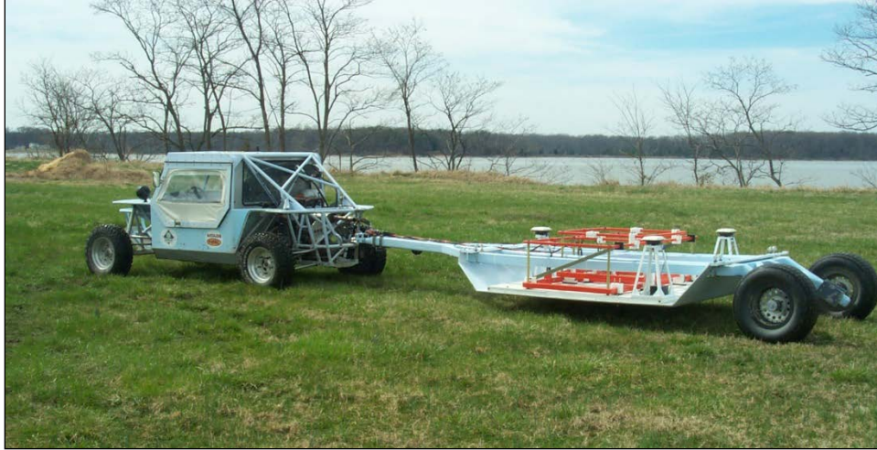
Figure 4-2 MTADS EM61 array pulled by the MTADS tow vehicle.
