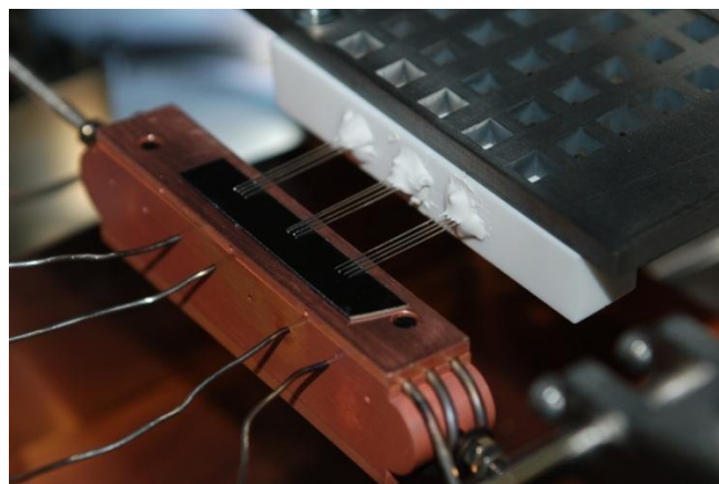
Figure 28: Photo of a sample positioned on the heater inside the vacuum chamber. 12 tungsten needles in groups of four are contacting the sample for 4-point resistance measurements. Also shown are the thermocouples inserted into the copper block of the heater.
