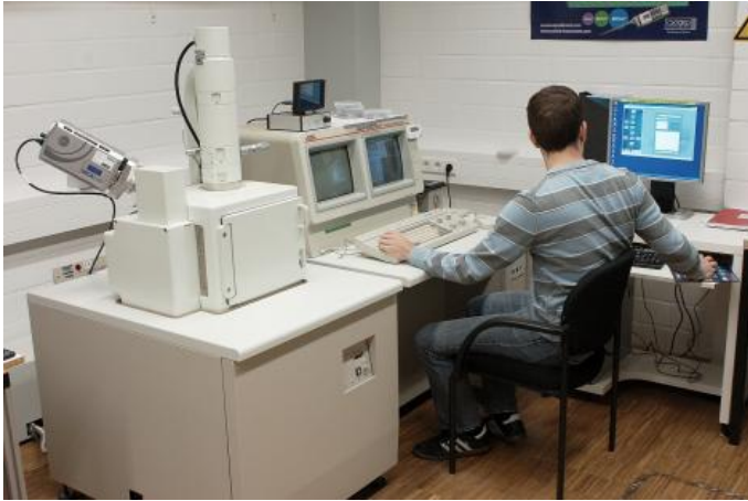
Figure 9: Scanning electron microscope with automated sample stage for composition mapping by energy dispersive x-ray spectroscopy.
