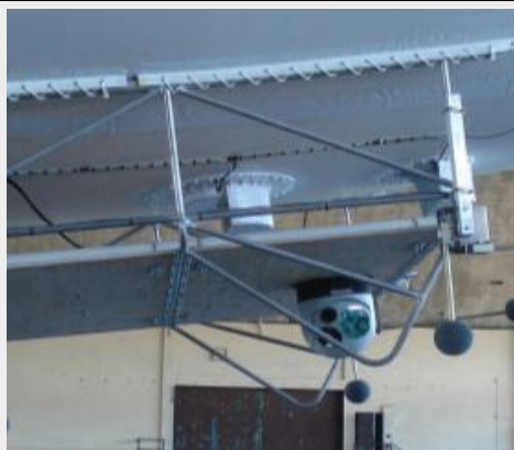
Figure 55: Payload Mounted On Airship; AWSS (left) and Gondola With MX-14 Turret (right) 54
