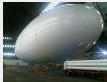
Figure 33: Inflated Envelope without Tail Fins 34
