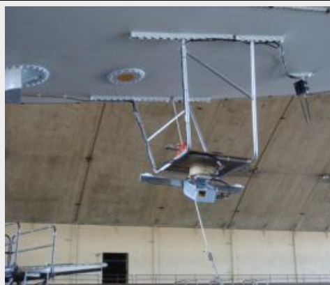
Figure 55: Payload Mounted On Airship; AWSS (left) and Gondola With MX-14 Turret (right) 54
