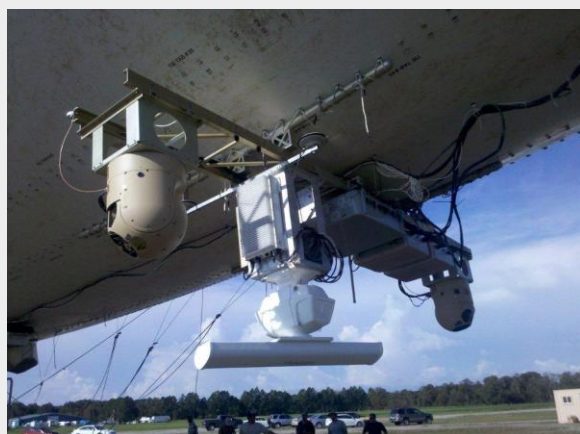
Figure 16: Underside of PGSS Showing Payload Support 24
