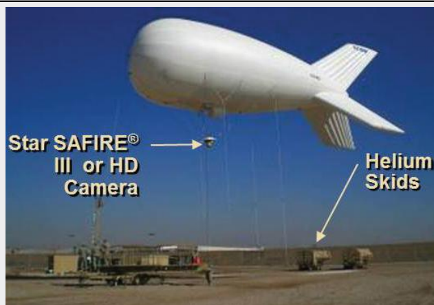
Figure 20: RAID Showing Payload and Ground Components 27
