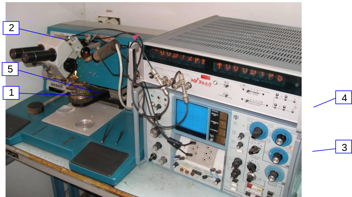
Figure 3. Photograph of the stand for characterization of metal-diamond-metal structure in the 25÷400°C temperature range
