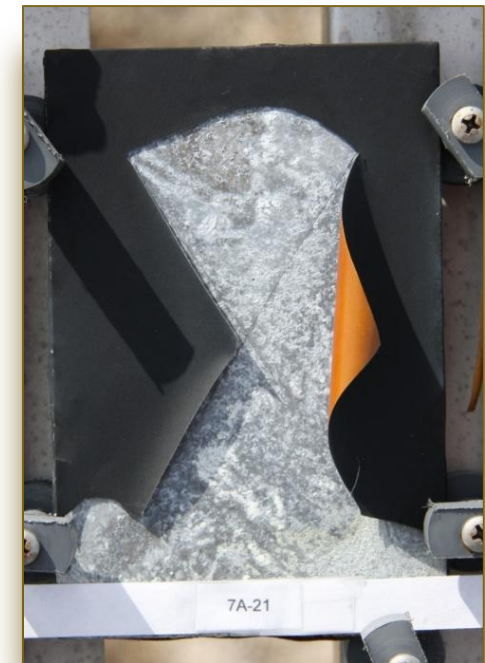
Conversion Coating B/ HT Resin Coating/ 23377C/53039
