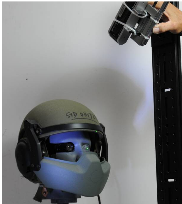
Figure 8. Objective assessment of the upper FOV. Height of laser adjusted to intercept edge of the helmet and pupil of the eye to determine upper FOV angle.
