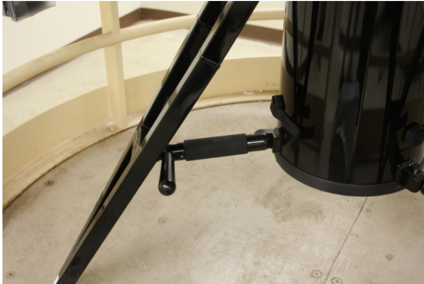
Figure 4.3 Stabilization strut onto PPR leg complete
