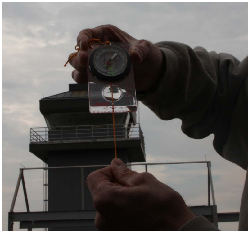
Figure 5.5 Mason's string tied to magnetic compass
