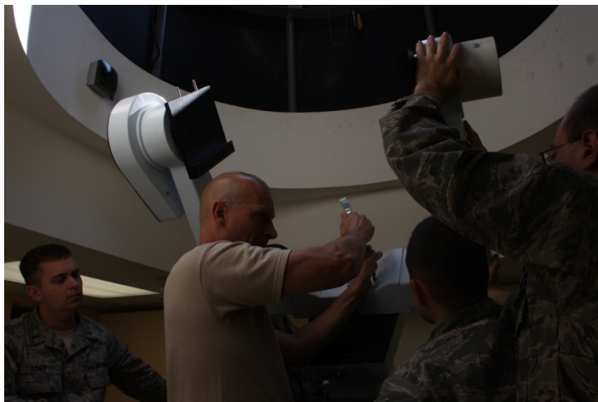
Figure 8.4 Securing the equatorial fork onto the polar assembly
