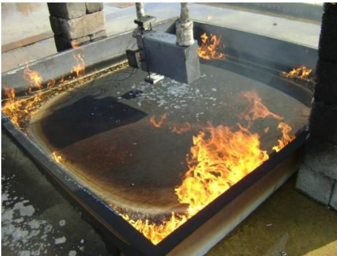
Figure 27. Photograph of condition of pan after test no. 1 conducted without water sub-layer present.
