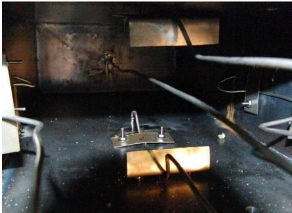
Figure 7. Photograph of thermocouples mounted on the interior surface of the containers as taken from the top looking into the container.
