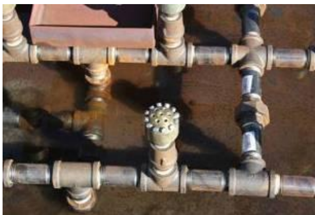
Figure 38. Photograph of spray heads to be used in propane area burner.
