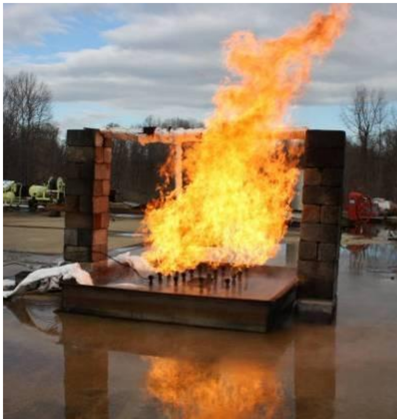
Figure 45. Photograph of propane area fire.
