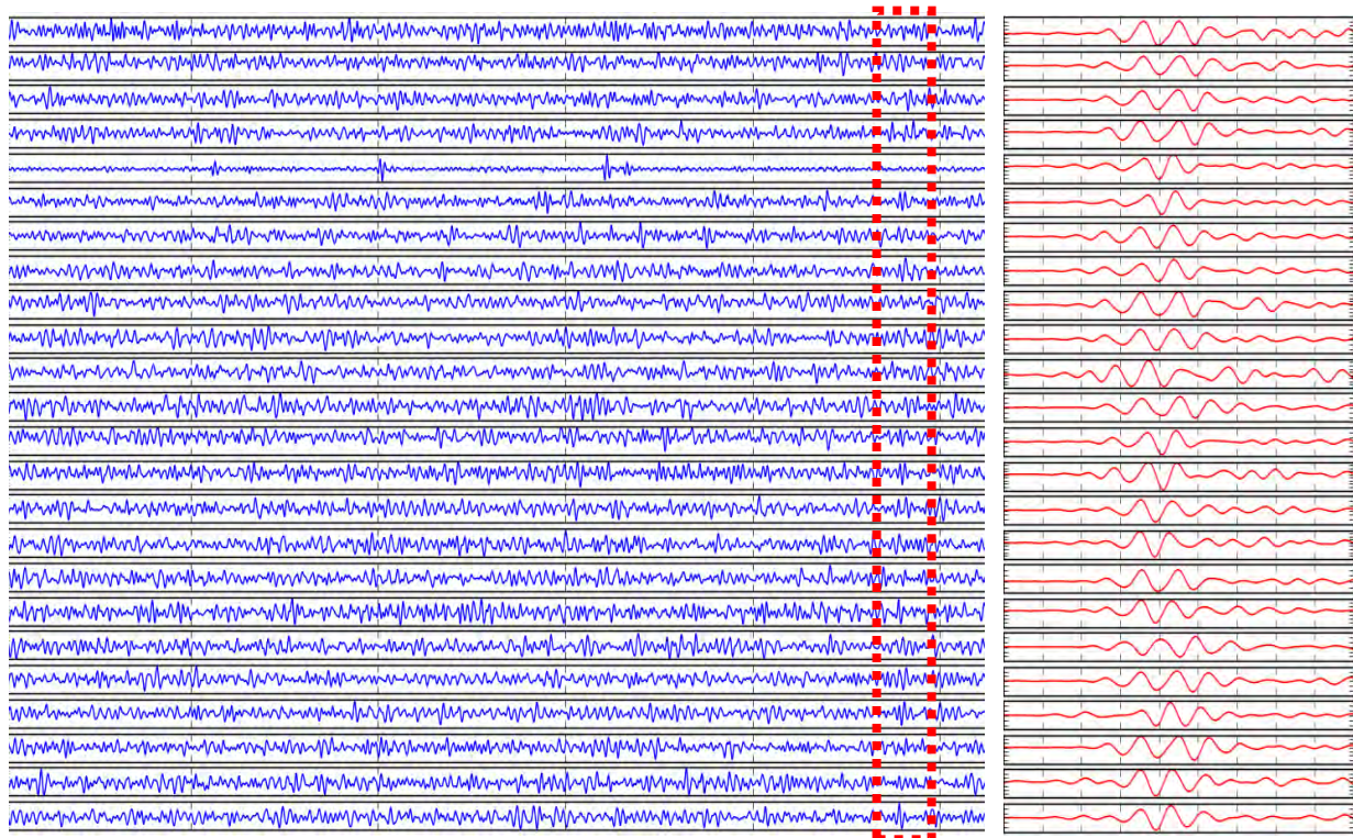
Figure 1. IMS seismic array PS2 (WRA). Waveforms recorded on vertical channels and an example of waveform template (right panel). One correlation coefficient is calculated over the entire template with all channels aligned in one record. In the template, individual channels are shifted in time according to theoretical travel time residuals defined by azimuth and slowness of the origin (source/receiver) beam. All waveforms are also shifted by the same time delays between individual channels. Hence, the empirical time delays between the channels are retained when the template is convolved with the waveforms.
