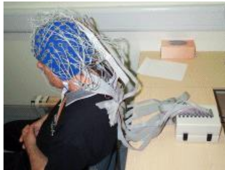
Figure 6. The 64-channel BioSemi EEG System (33).
