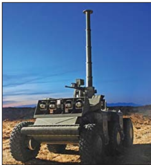
Crusher vehicle with payloads: a stabilized remote weapons station and an extended RSTA mast.
