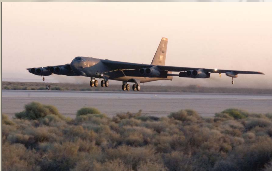
A B-52H aircraft successfully demonstrated an eight engine flight test with a Fischer-Tropsch and JP-8 Blended fuel mixture.
