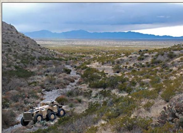
Crusher vehicle autonomously navigating through a dry wash at Ft. Bliss, Texas
