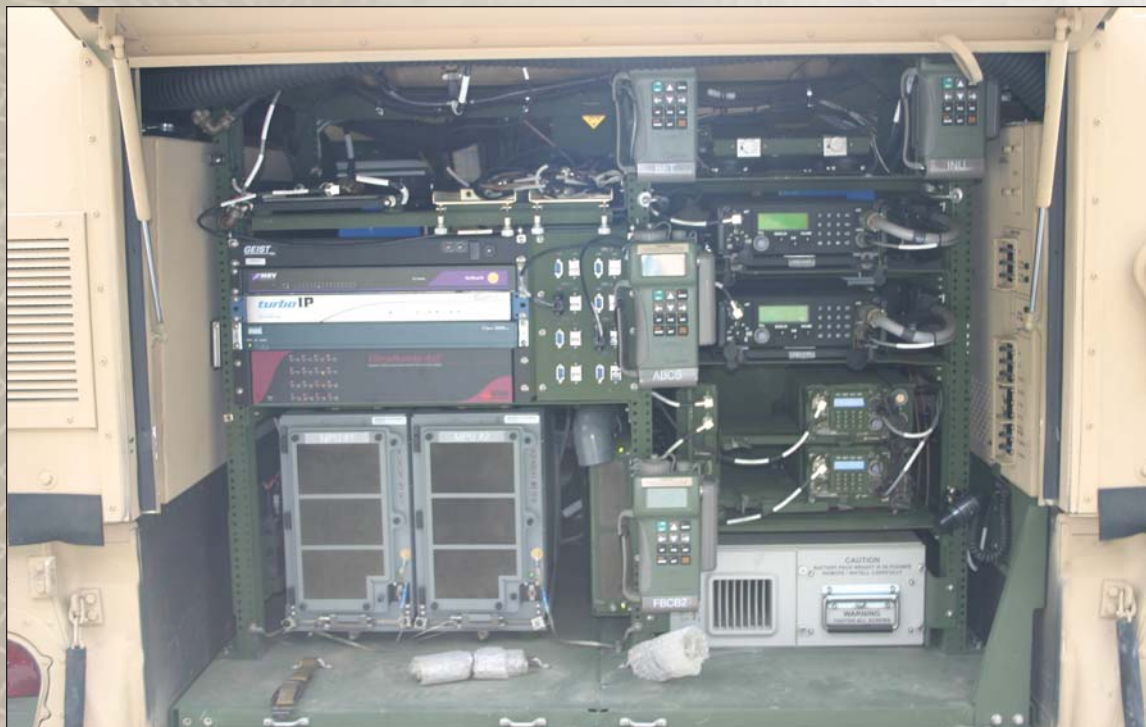
MBCOTM PP1 HMMWV variant, rear view of the C4ISR mission equipment showing the dual 4 slice Multi-Processing Unit, communications and networking equipment
