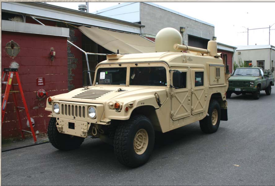
MBCOTM PP1 HMMWV variant, external view with the KU-Band on the Move antenna system
