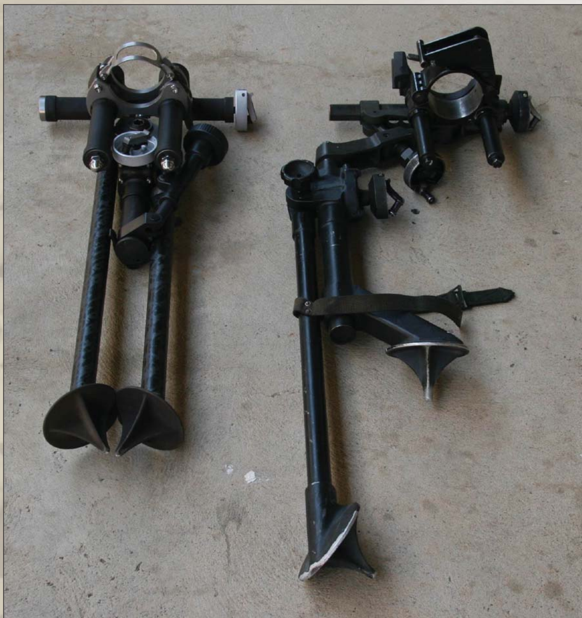
The LW81mm bipod packs up smaller than the currently fielded bipod and is easier to transport.
