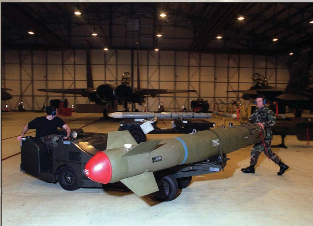
U.S. Air Force Senior Airman Paul Kaehler (left) and USAF Staff Sergeant Barry Mueller, weapons loaders from the Weapons Standardization Section, 48th Operations Group, 48th Fighter Wing, Royal Air Force Lakenheath, United Kingdom, prepare to load an advanced EGBU-15, a guided air-to-surface weapon on an F-15E Strike Eagle aircraft.
