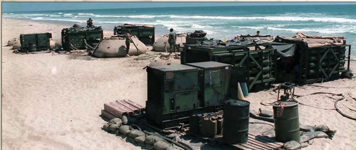
Reverse osmosis equipment
