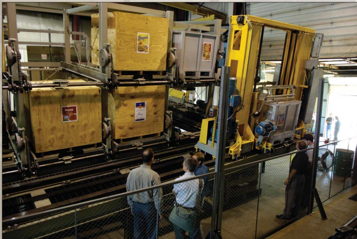
ASRS Demonstrator on 3.5° pitch / 8°roll platform for land-based testing
