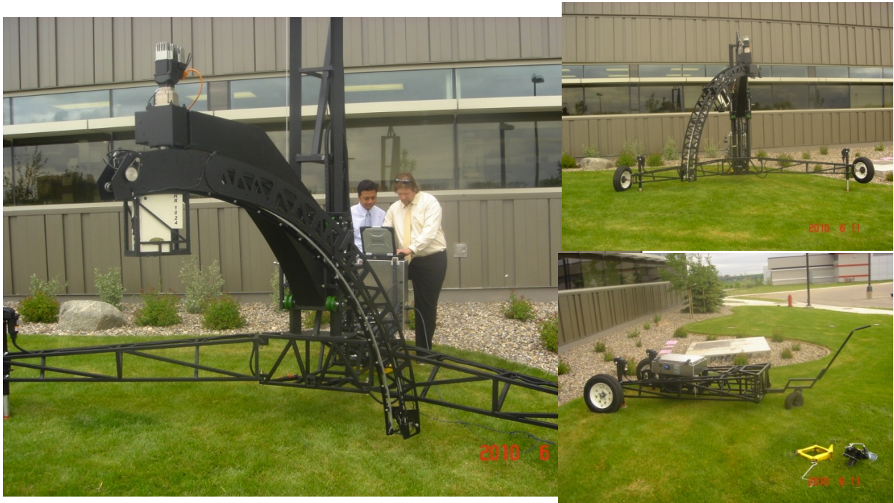
Figure 45. The NRL Goniometer for Outdoor Portable Hyperspectral Earth Reflectance (GOPHER) was acquired under a capital equipment purchase in July 2010. Developed by SpectraVista, University of Lethbridge, and the University of Saskatchewan, this goniometer is capable of characterizing the bi-directional reflectance distribution function (BRDF) which characterizes hyperspectral reflectance over a full hemisphere with a portable full-range (visible, near infra-red, and short-wave infra-red) HR-1024 spectrometer. BRDF can vary dramatically with sun-target-sensor geometry, and multi-angular studies will allow improvements in the extraction of important environmental parameters.
