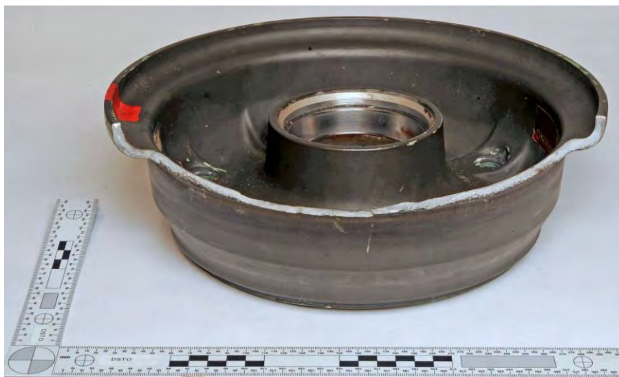
Figure 1. Photograph of the wheel following removal of the tyre. A section comprising approximately one third of the circumference had separated from the wheel at the bead seat.
