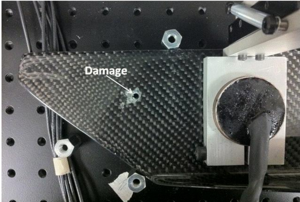
Figure 8.36. Damage introduced to the composite test sample.
