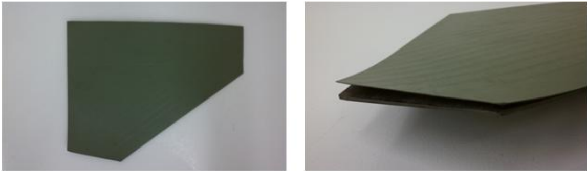
Figure 6.5. An Air Force composite panel with a delamination defect located at one corner of the panel.
