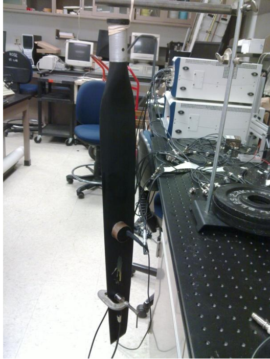
Figure 8.41. Experimental setup for the initial tests on a composite propeller blade.
