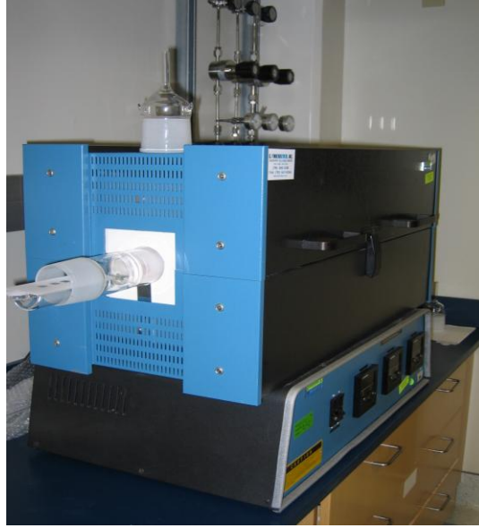
Figure 4. Three zone furnace used for curing BSTO films.
