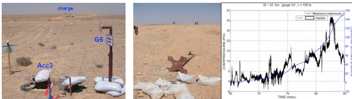
Figure 6. The most remote co-located accelerometer Acc3 and pressure gauge G6 at 611 m (left). The closest gauge G1 at 109 m after the explosion (center) and the record (right)
