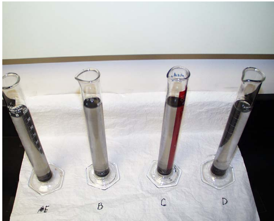
Figure 8. Carbon settling Test II- 900 minutes (A: TIGG 5D; B: GC Powdered; C: WPX-D; D: WF-PAC-600).
