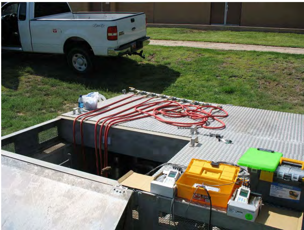
Figure C2. Compressed air distribution manifold and data acquisition equipment.
