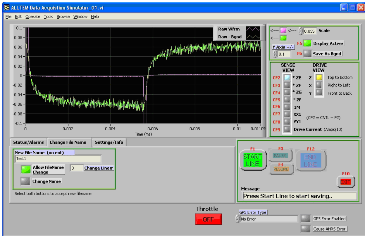
Figure 5.7. The Change File Name tab, lower left of screen, allows the operator to choose another file name for storing subsequent data.
